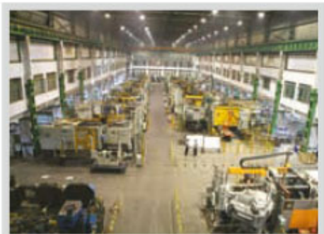
Comprehensive range of HPDC equipment ranging from 160T to 3200T locking force
