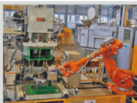
Completely integrated cells with robotic extraction, auto-sprayers, dosing furnaces, and integrated trimming presses.
